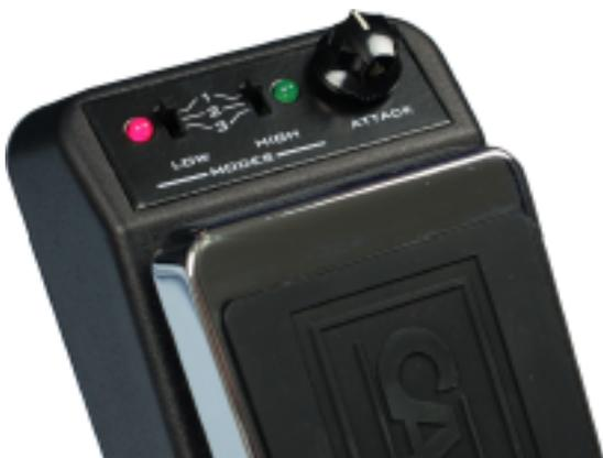
Select position 1, 2, or 3 in both High and Low Modes, engage the effect and fine-tune the attack of this effect by adjusting the Attack knob (also on the front of the 2 Wah). The green (Low) and red (High) LED's indicate which Mode you are in, with Low being typically for lead work, and High being used more often for rhythm work.
