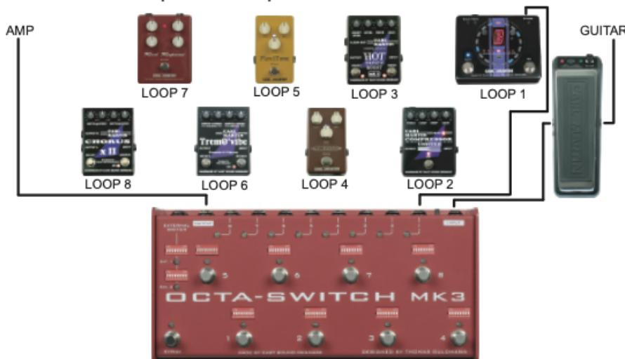
Connect a tuner to i.e. loop 1 send, and nothing in the loop return, select i.e. program 8 with only loop 1 engaged, this way you mute the system while getting signal to your tuner, without the signal passing through the tuner.
